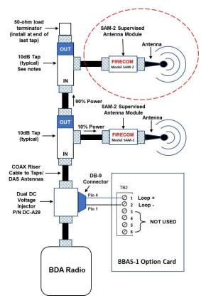
The signaling between the BBAS-1 and the supervised life-safety antennas must pass properly through the passive coaxial radio distribution wiring and splitting devices. A fault in any of the intermediary devices or pathways results in one or more antenna communication troubles to be detected.
