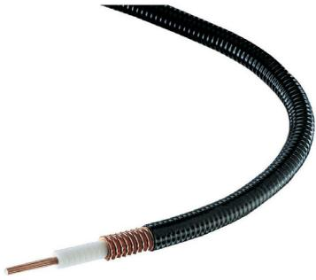
FSJ4RK-50B, HELIAX® Superflexible Foam Coaxial Cable, corrugated copper, 1/2 in, black non-halogenated, fire retardant polyolefin jacket B2ca-sla-d0-a1 (CPR testing is conducted annually please reference the website for latest classification)
